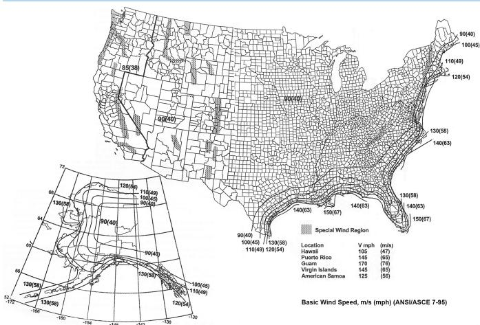
The Effective Projected Area (EPA) standards shown in the Load and Dimensional Data Tables on the specification sheets are designed to withstand dead loads and theoretical dynamic loads developed by variable wind speeds, as charted, with an appropriate wind gust factor under the following conditions:
