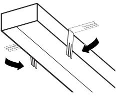
Hand bend outer tabs on the SRK brackets around the fixture housing sides to keep SRK brackets in the desired position.
