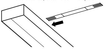
STEP 2: Center brackets on the fixture housing.
