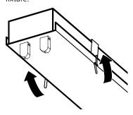
STEP 7: Confirm correct lamp orientation on sockets based on fixture "N", "L" marking. Make sure the lamps are correctly seated in the lampholder (sockets) before twisting.
