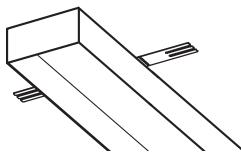
STEP 3: Hand bend both ends of SRK brackets downward.
