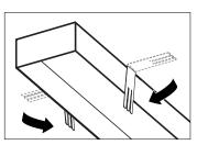
**STEP 5:** Hand bend outer tabs on the SRK brackets around the fixture housing sides to keep SRK brackets in the desired position.
