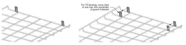
2. Attach the clips to the end plates of the fixture using #8 screws supplied.
