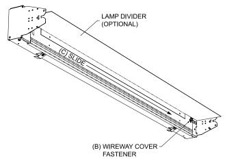
STEP 3: Mount the fixture channel to the wall using fasteners (furnished by others) appropriate for the mounting surface. Various electrical K.O.'s and mounting holes are provided for supply wire entry and mounting to the wall (refer to illustrations below).
