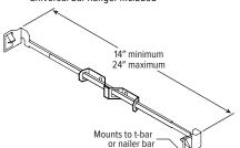
**BA1M** Adjustable butterfly pan bracket, aluminum, bar hanger not included (N Mounting Type only)
